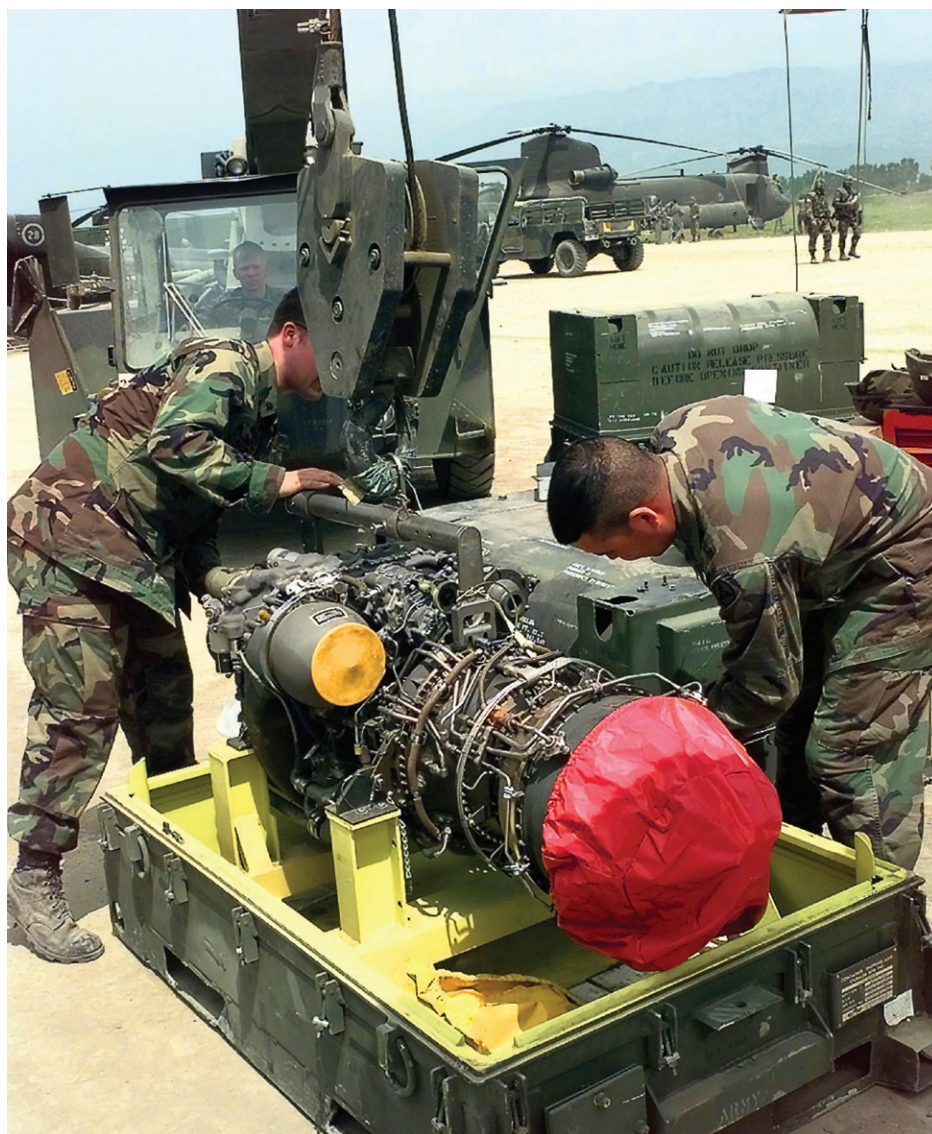
Army aviation mechanics prepare to perform maintenance on a servo mount of a T-700 engine of a Black Hawk helicopter, while deployed to Albania in support of Task Force HAWK.
