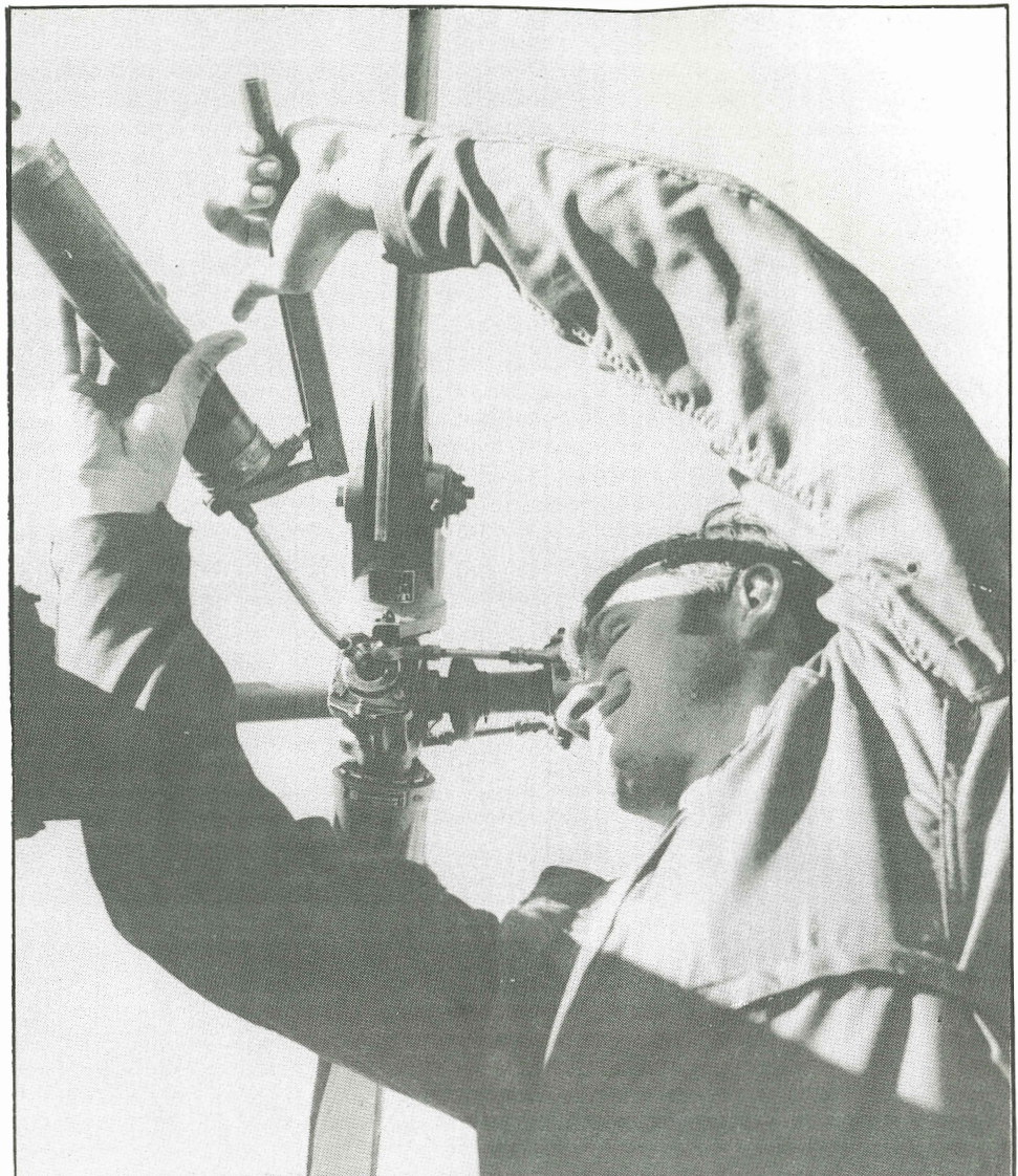
SGT. JERRY WATKINS , Detachment 1, 1155th Transportation Company, Frankfort, services the tail rotor of a UH1H helicopter. (Photo by Sgt. Danny Sexton, 1155th Transportation Company, Frankfort, and managing editor of the JOHNSON COUNTY JOURNAL , Paintsville.)
