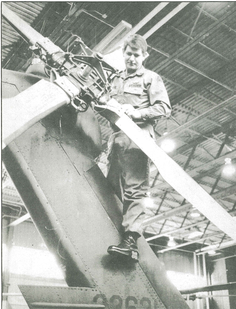
SFC BO THOMAS checks the tail rotor on the UH-60A Blackhawk. Visual inspections like this are conducted every seven days. (Photo by Spec. 4 Ed Armstrong)
